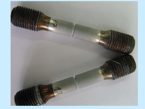
Hydrogen embrittlement test: 4340 steel coated by Zn-polymer coating is not susceptible to hydrogen embrittlement
