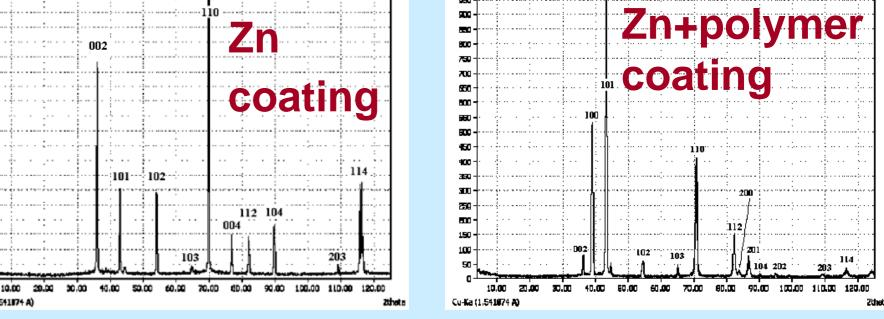
• Wider diffraction lines of sample with organic additive at (110) are a consequence of the smaller grain size.
