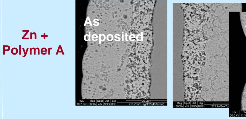
**Zn+ polymer B coating is less dense than Zn+ polymer A** coating, and as a result does not crack during heat treatment
