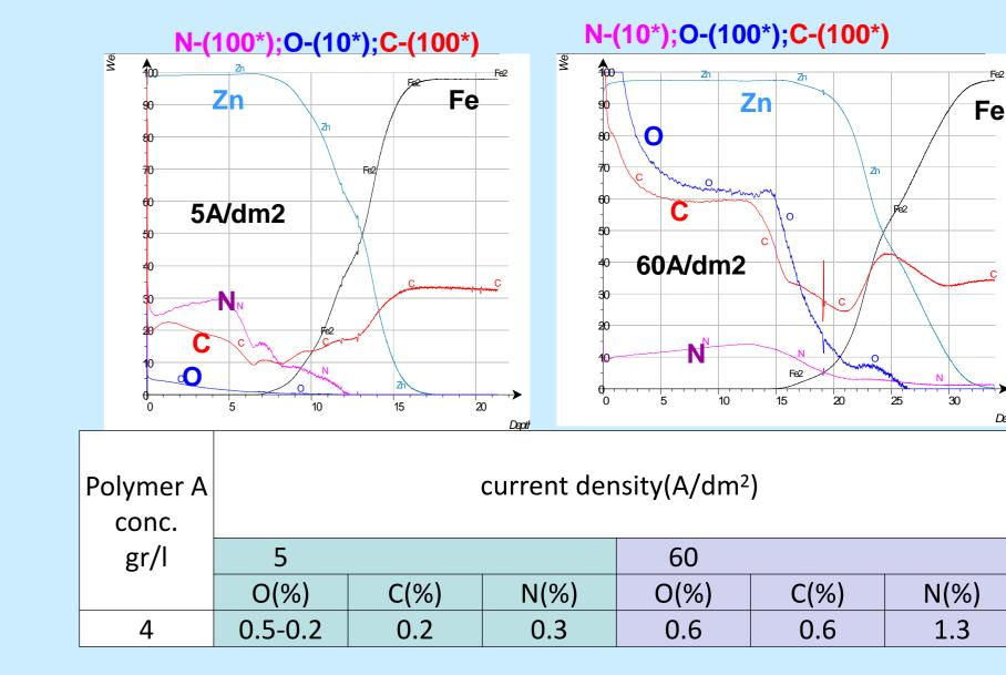
**Increase in current density resulted in increase in** polymer content in Zn coating
