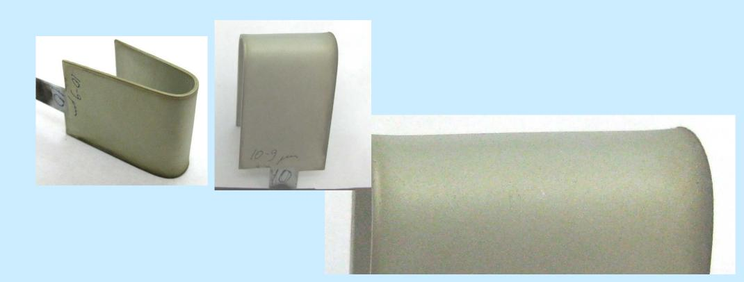
Adhesion test: A very good adhesion of the Zn-polymer coating on 4340 steel
