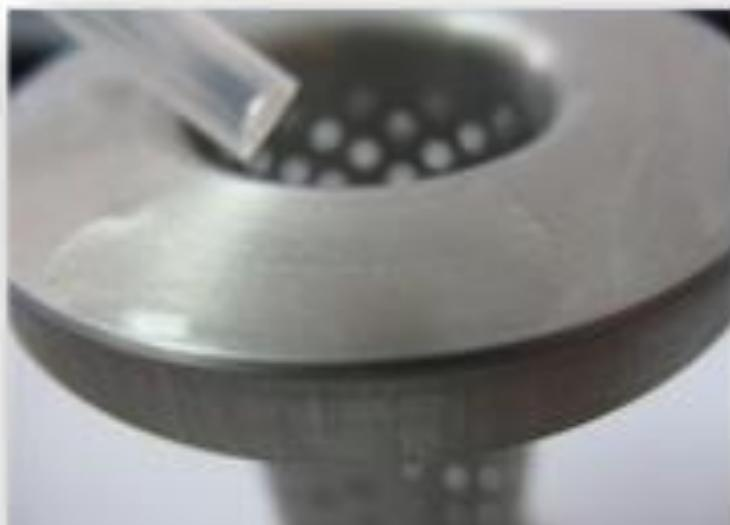
Image of water drop on Al6061 surface before coating
