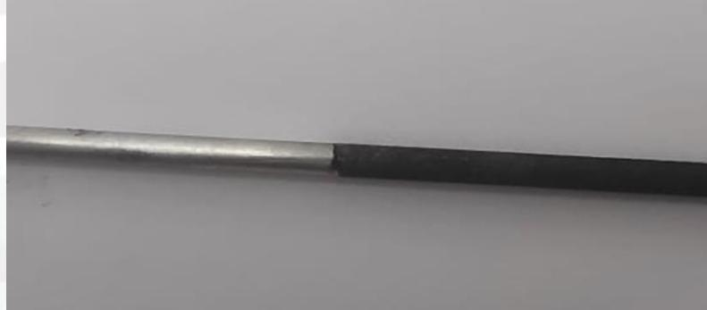
Electrophoretic deposition of ceramic coatings
